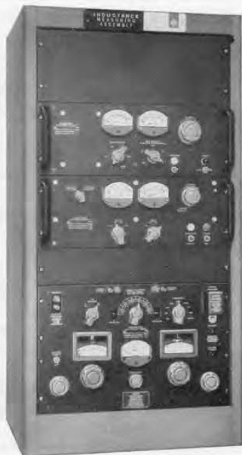
Figure 1. View of the Type 1630-AL Inductance Measuring Assembly. Space is provided at the top of the rack for the addition of an oscilloscope, which permits the current waveform or the hysteresis loop to be viewed during the measurements.
